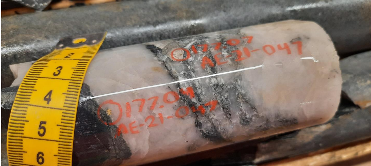
Figure 1: Core photo showing multiple occurrences of visible gold in drill core from AE-21-047 at a depth of 176.70m – 0.8m sample graded 19.4 g/t Au.
