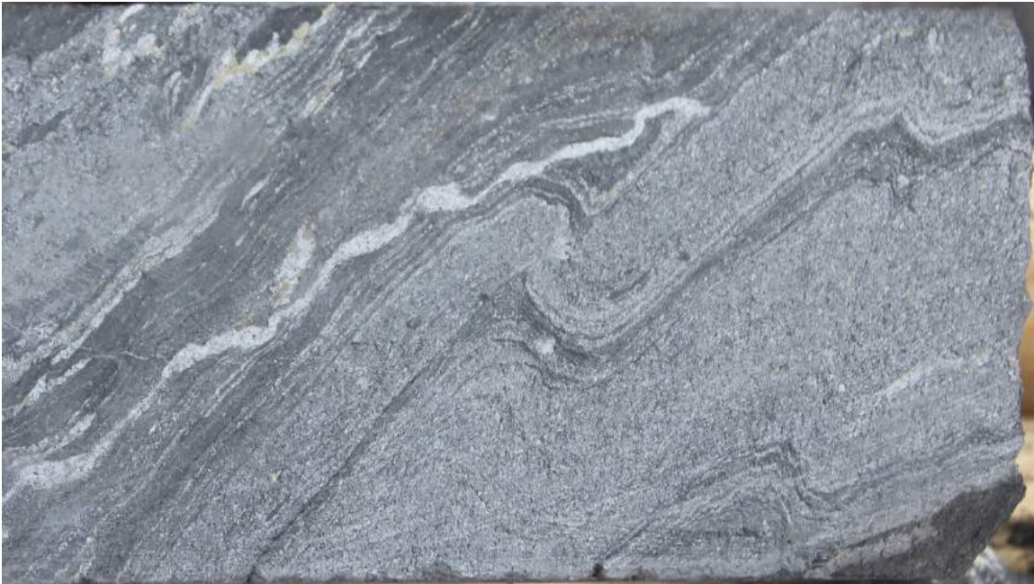
Figure 3. Z-shaped drag fold in NQ (~5 cm diameter) drill core from Mikwam. This structure is reflective of the significant regional structures.
