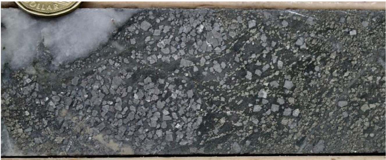
Figure 2. High grade zone intersected in hole AUL-19-30 at 206m depth with typical coarse arsenopyrite and pyrite. Late stage quartz vein cuts mineralization in upper left of image.
